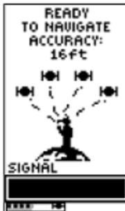
A good initial activity is to turn the handheld unit on and get students to observe the initial page which shows the unit acquiring a satellite.
